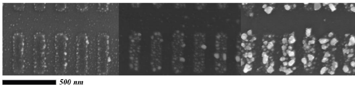
Figure 11: SEM micrographs of patterned nanorods on a glass
