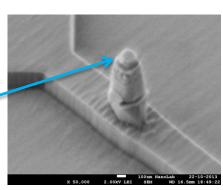
Additional lithography step to protect pillar with photoresist
