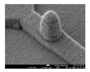
Unprotected pillar due to mask erosion
