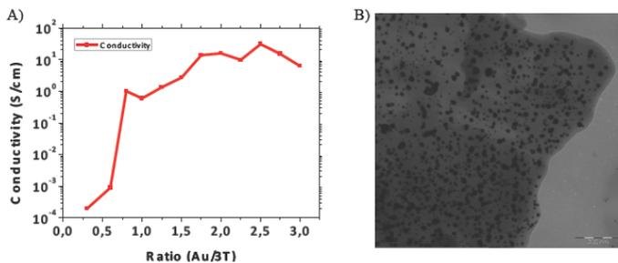
Figure 2: A) Dependency of IPN conductivity on Au/3T molar ratio. B) TEM image of the nanocomposite
