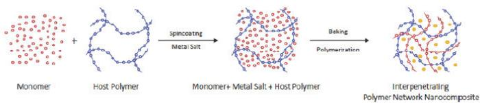
Figure 1: Scheme of in-situ synthesis of the conducting polymer and gold nanoparticle in a host polymer.
