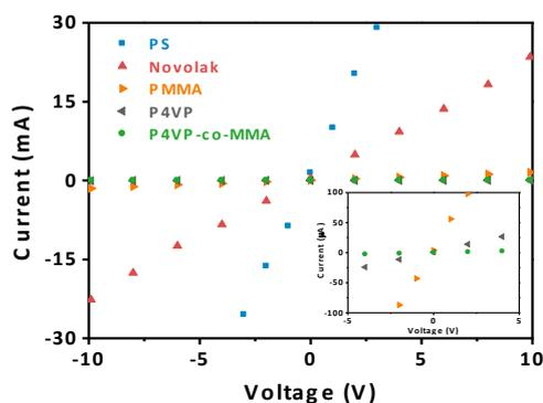
Figure 2: I-V Characteristics of conducting IPN films prepared from different host polymer.
