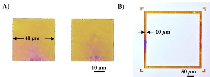
Figure 1: Examples of micropatterns of novolak-based conducting polymer fabricated by means of photolithography
