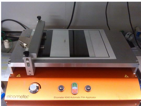
Fig. 2: Doctor-blading equipment for the QD film formation.
