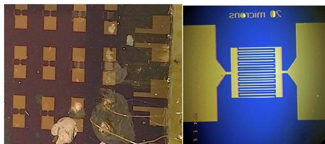
**Fig. 5.** Photograph of interdigitated photoconductors with a QD-layer on one of them and zoom image of one of them (20 μm gap).
