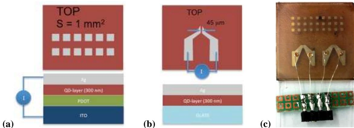
**Fig. 4.** Schottky/heterostructure photodiodes (a) and micro-gap photoconductor (b). Mask used for the Ag electrode deposition is the same for both designs (c); in the example contacts are made on the photoconductive design.
