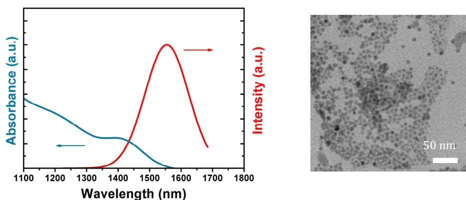
**Fig. 1:** Absorption and PL spectra (left) and TEM image (right) of oleylamine-capped PbS QDs in octane (left).
