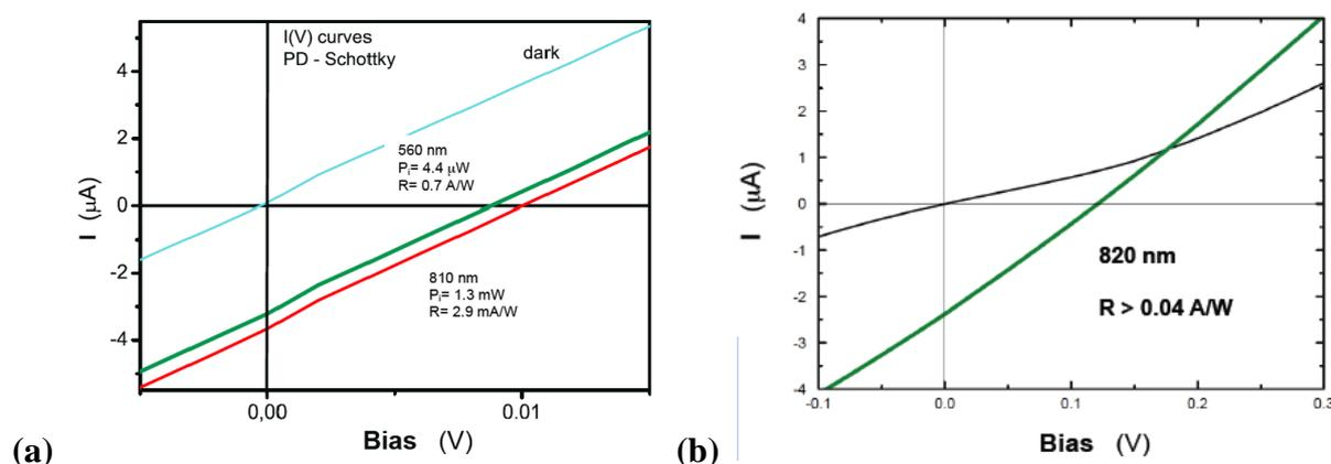
**Fig. 6.** Comparison of the I(V) characteristics of the best ITO/PDOT/PbS-QD-solid/Ag photodiodes: spin-coating (a, from previous report) and doctor blading (b). The QD-film thickness is very similar in both devices (360 nm).
