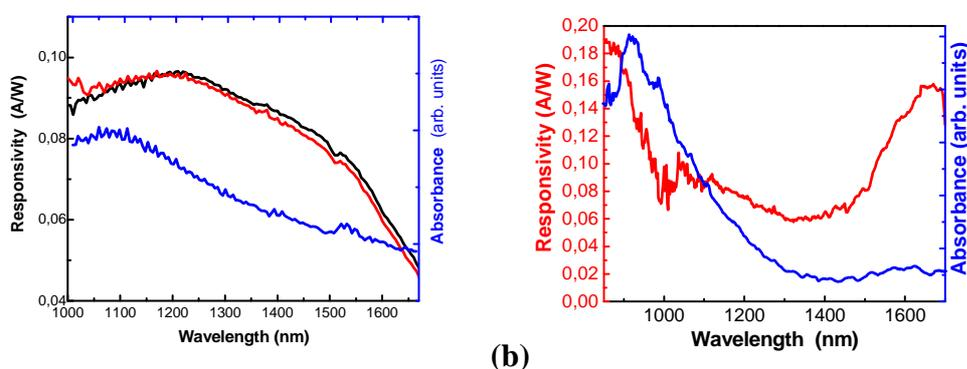
**Fig. 8.** Responsivity spectra for the first (a) and second (b) generations of glass/ITO/PEDOT/QD-film/Ag photodiodes (black and red curves in **a** and red curve in **b**) where the QD-films (300 and 500 nm for **a** and **b**) were prepared by Dr-blading and the corresponding absorbance spectra (blue curves).
