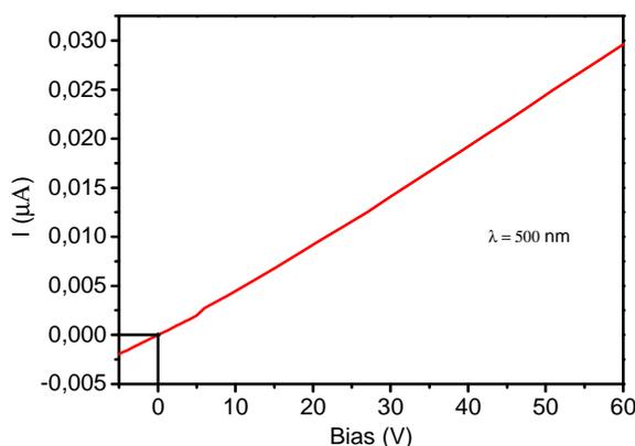
**Fig. 7.** I(V) characteristics of a microgap PbS-QD-solid(500 nm)/Ag photoconductor produced by doctor-blading and Br<sup>-</sup> to replace the original oleylamine ligands.
