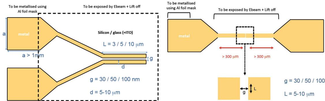
**Fig. 10.** Fabrication layouts for the fabrication of nanogap plasmonic waveguide photoconductors. In dotted area is indicated the fabrication by using ebeam lithography.
