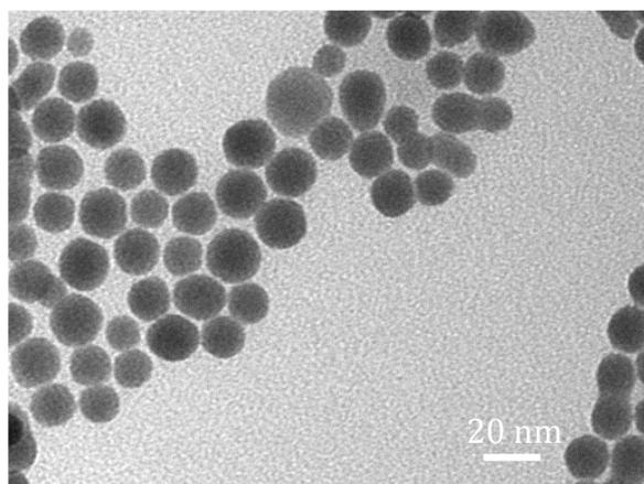
**Fig. 3.** TEM image of  $\text{Ag}_2\text{S}$  colloidal QDs.
